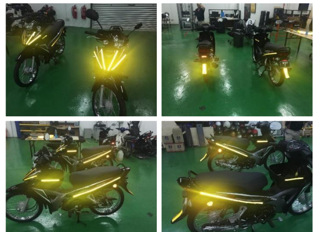
Figure 1: Yellow-coloured Diamond Grade Conspicuity Markings Series 983 applied on two motorcycles [also visible are the rear and side reflex reflectors as mandated per regulation].
